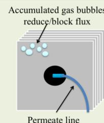
Figure: Schematic of trapped air in membrane modules.
