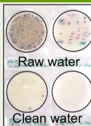
Figure (above): Examples of EC compact dry plates from membrane tank (raw water) and permeate (clean water) samples. Blue colonies are the number of *E.coli* and the sum of the blue and red colonies is the total coliform count.
