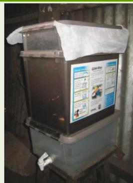
Figure: Prototype I of household gravity driven membrane filter.
