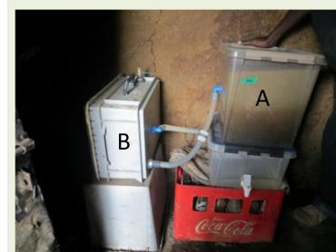
Figure: Assembled experimentation filter. Part A is the current prototype where the membrane is regularly exposed to air. Part B is a air and water tight tank where the membrane is continuously submerged in water. Both membrane tanks share the same raw water and clean water tanks.
