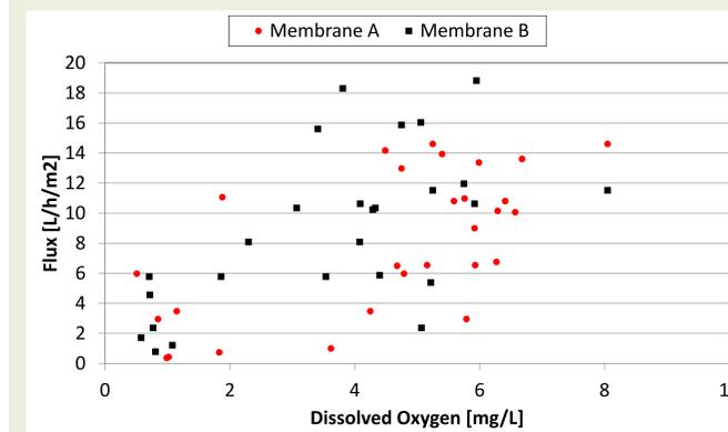
Figure: Correlation between dissolved oxygen and flux in the two different membrane module configurations. Membrane A is the current system and Membrane B is a submerged membrane system.
