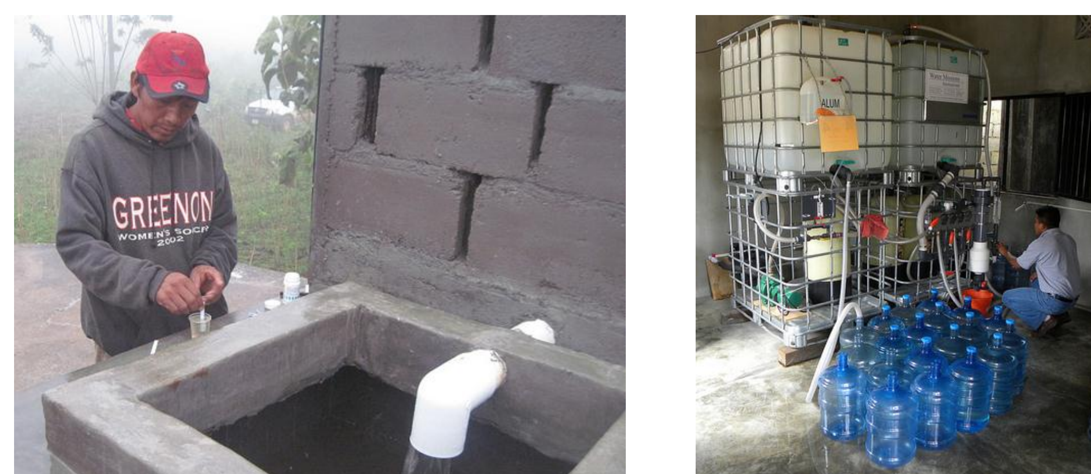
An operator of a water system in Honduras tests the free chlorine concentration in treated water (left); water system operators in Indonesia monitor a water meter while filling bottles for distribution (right)
